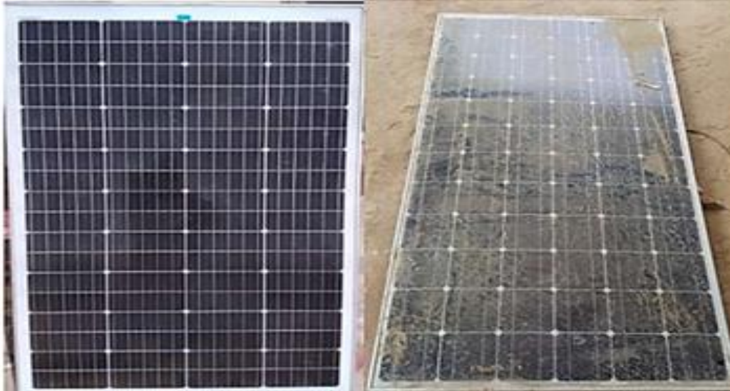
Fig. (2): Solar PV panels. a. Clear panel. b. Dusty panel
