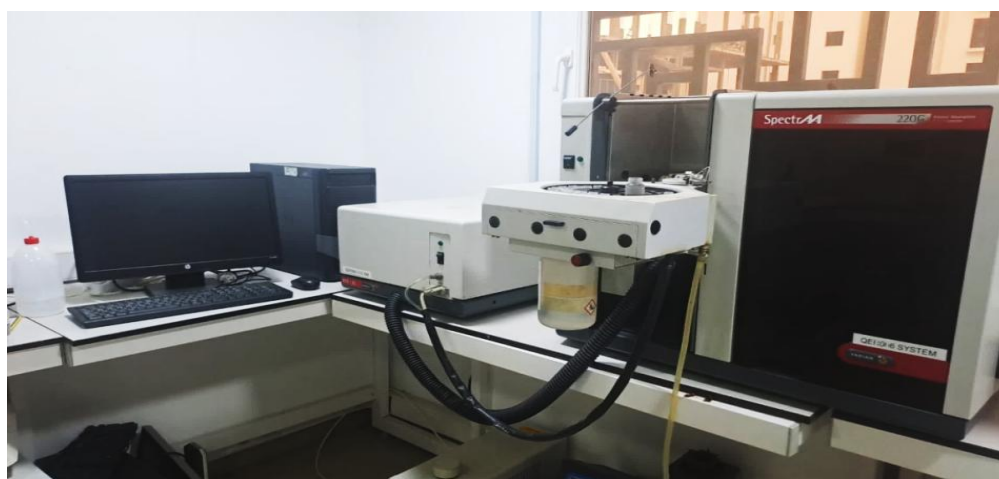
Fig. (6) Atomic Absorption Spectrophotometer setup used for heavy metal determination.
