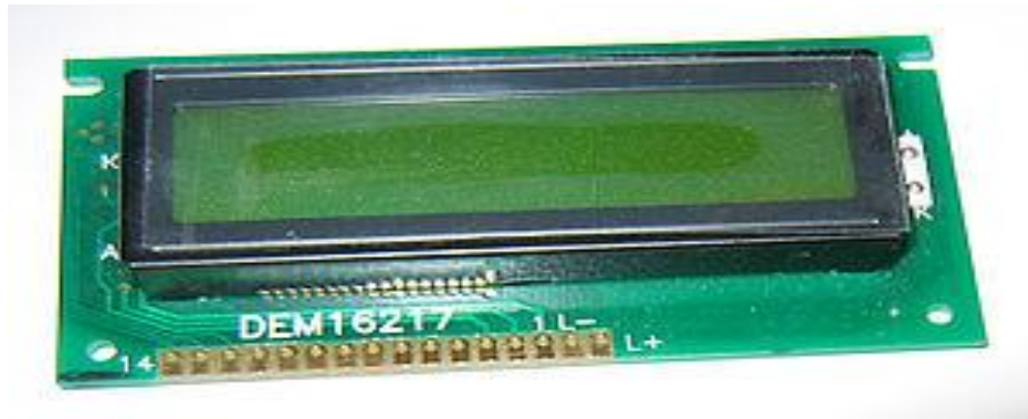
Figure (13): A general-purpose alphanumeric LCD, with two lines of 16 characters
