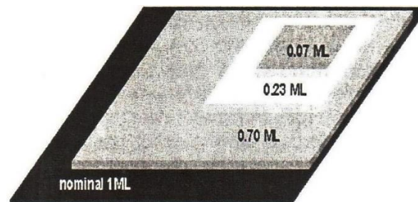
Figure 7. Model of a solid on solid-like film, based on the relative contribution of the spectral components resulting from the Fe monolayer 80K CEMS spectrum fit.
