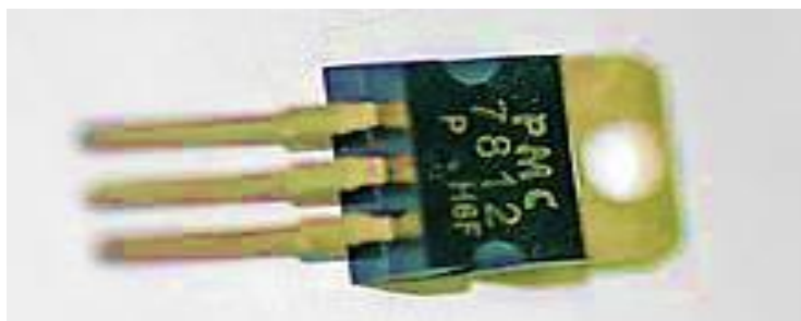
Figure (4): Voltage regulator
